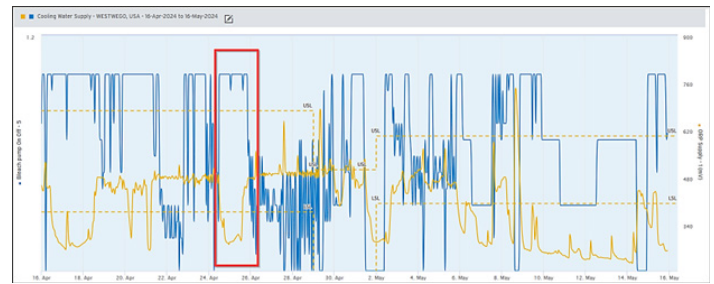
FIGURE 4: On 24-25 April, oxidation-reduction potential (ORP) declined, but the bleach pump relay indicated the pump was running. However, the bleach pump had failed. Once the pump was repaired, ORP increased and the deposit risk index declined, indicating a clean-up of the biofilm.
